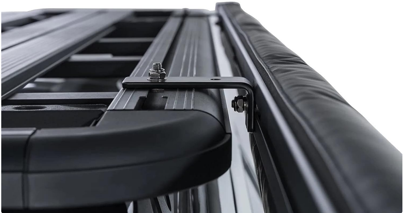
Image: Close-up of the mounting bracket installation on the roof rack.
