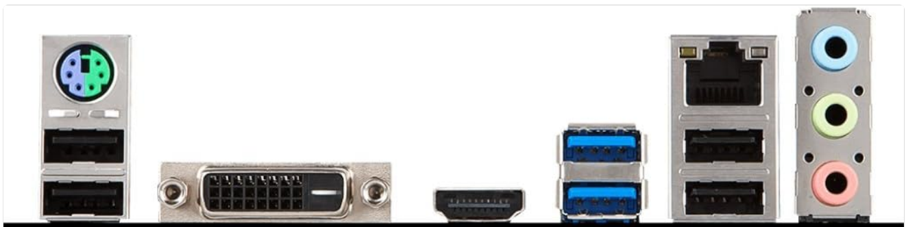
Figure 4.3: The rear I/O panel of the MSI H310-A PRO motherboard, showing ports such as PS/2, USB 2.0, DVI-D, HDMI, USB 3.1 Gen1, LAN, and audio jacks.
