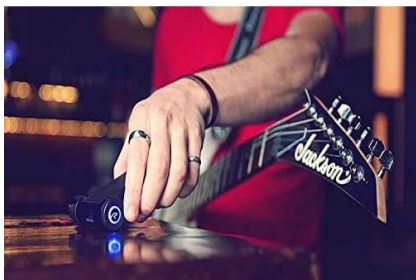
A user demonstrating how to attach the Roadie 2 to an electric guitar's tuning peg for automatic tuning.
