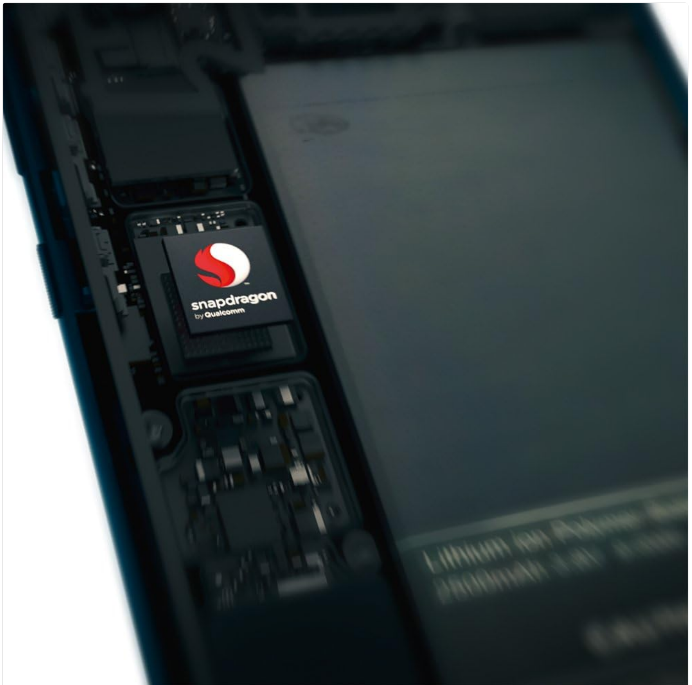
Figure 7: Internal view of the Moto G6 Plus, highlighting the Qualcomm Snapdragon processor.
