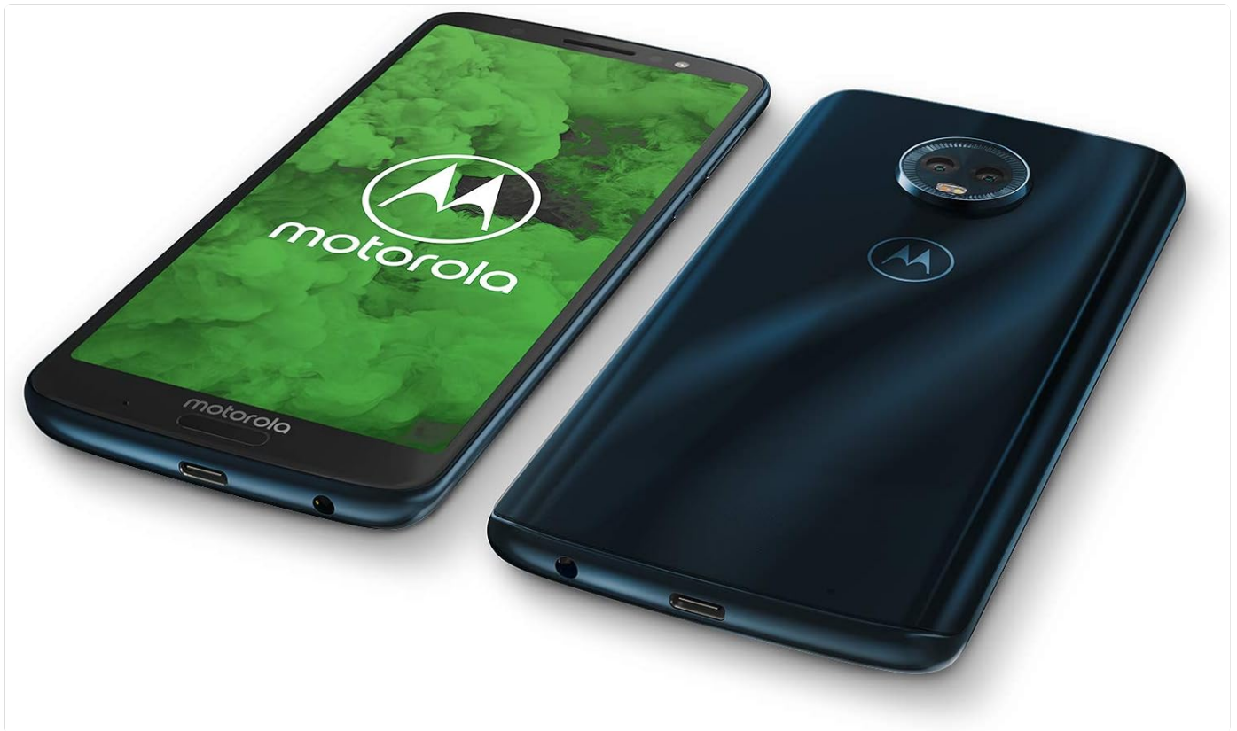
Figure 4: Bottom view of the Moto G6 Plus, illustrating the USB-C charging port and 3.5mm headphone jack.
