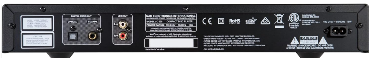
Image: Rear view of the NAD C 538 CD Player, showing the digital and analog audio outputs, and power input.
