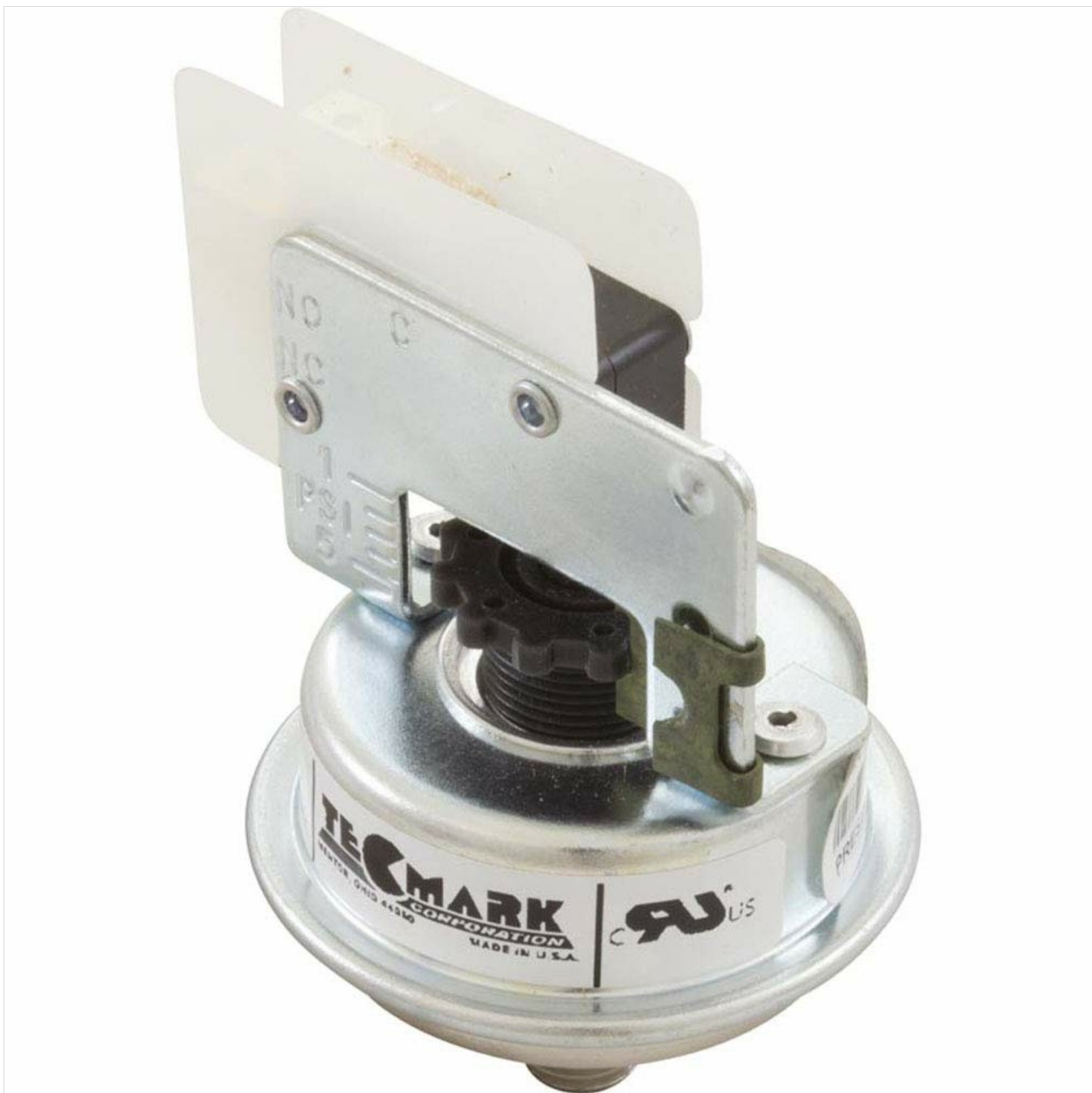
Figure 3.2: Side view of the pressure switch, highlighting the electrical terminals labeled NO (Normally Open), NC (Normally Closed), and C (Common). This model is SPST, typically using C and NO.
