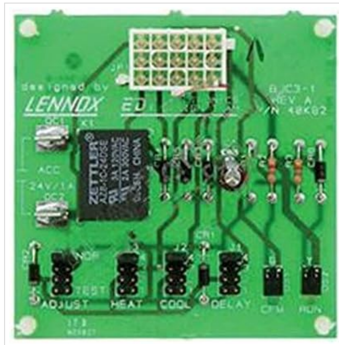
Figure 1: Lennox 40K82 BDC3-1 Circuit Board. This image displays the green circuit board with various electronic components, connectors, and labeled jumper settings for configuration.
