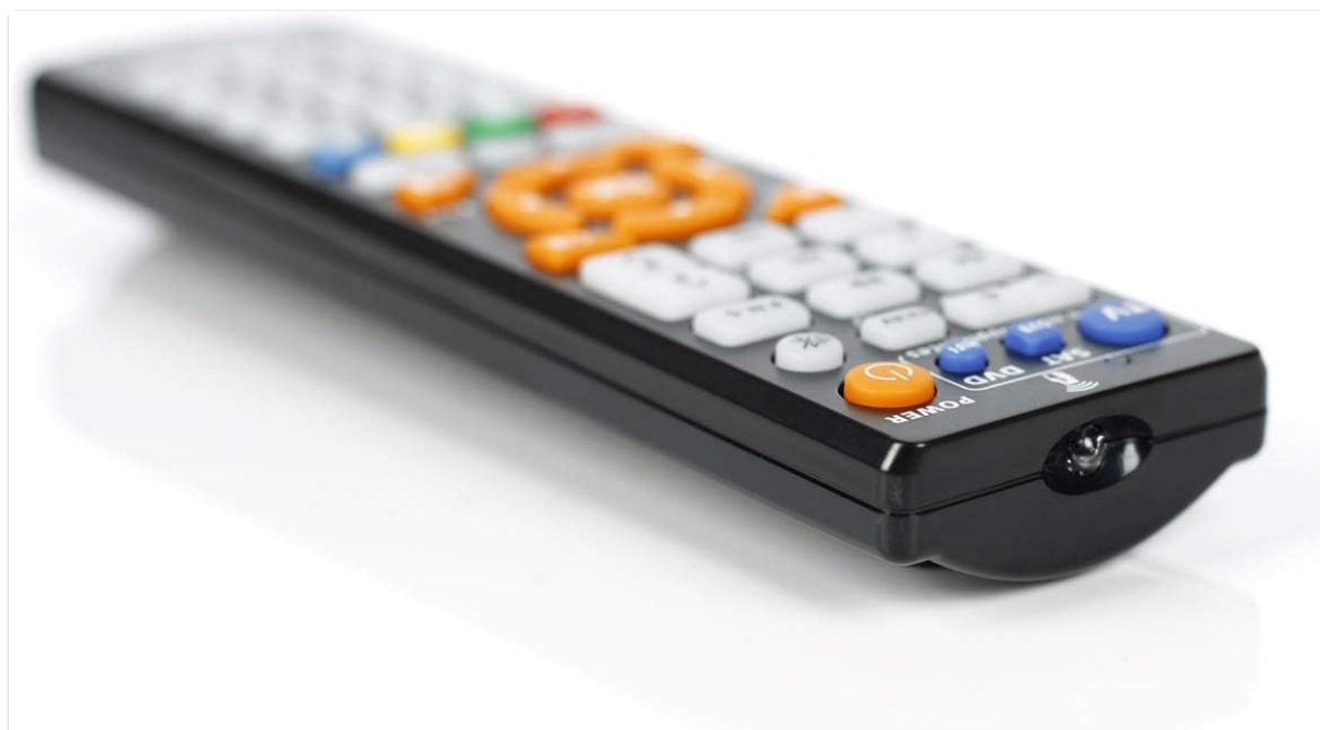
Image: A side view of the CHUNGHOP L336 remote control, highlighting the infrared (IR) emitter at the front.
