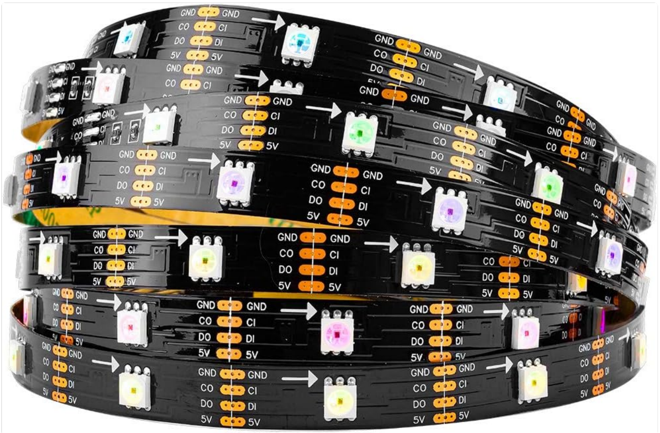
This image displays the BTF-LIGHTING SK9822 LED strip, coiled to show its flexible black PCB and the individual LED chips with their data and clock connections.
