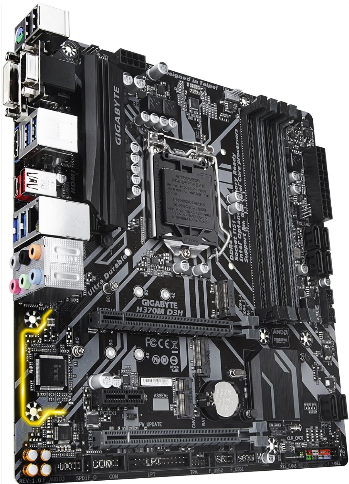
Figure 4.2: Angled view of the GIGABYTE H370M D3H Motherboard. This perspective highlights the PCIe expansion slots and the general layout of the board's components.
