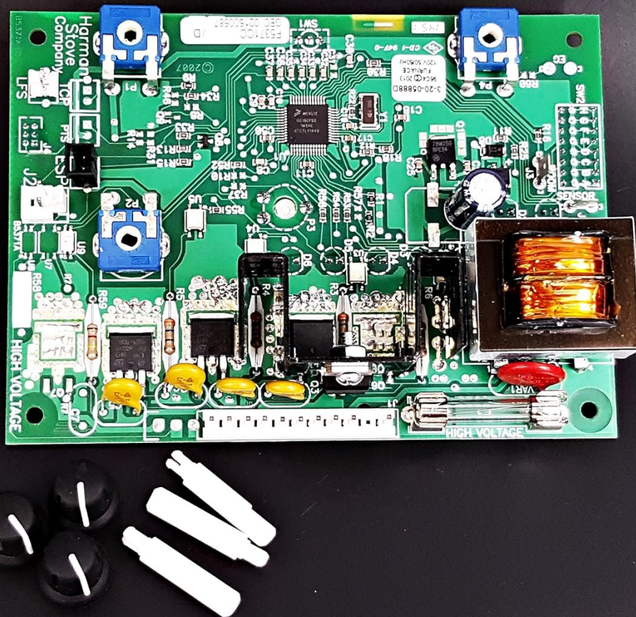
Figure 1: The Harman PF100 & PF120 Control Board (Model 1-00-05888) shown with accompanying control knobs and mounting standoffs.
