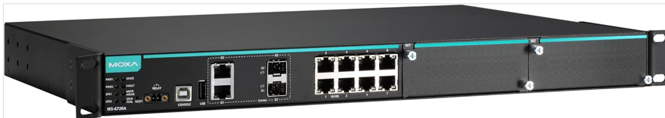
Figure 1: Front view of the MOXA IKS-6726A-2GTXSFP-HV-T Modular Managed Ethernet Switch, showing the 8 x 10/100BaseTX ports, 2 x 10/100/1000BaseTX or 100/1000BaseSFP combo ports, console port, USB port, and LED indicators.
