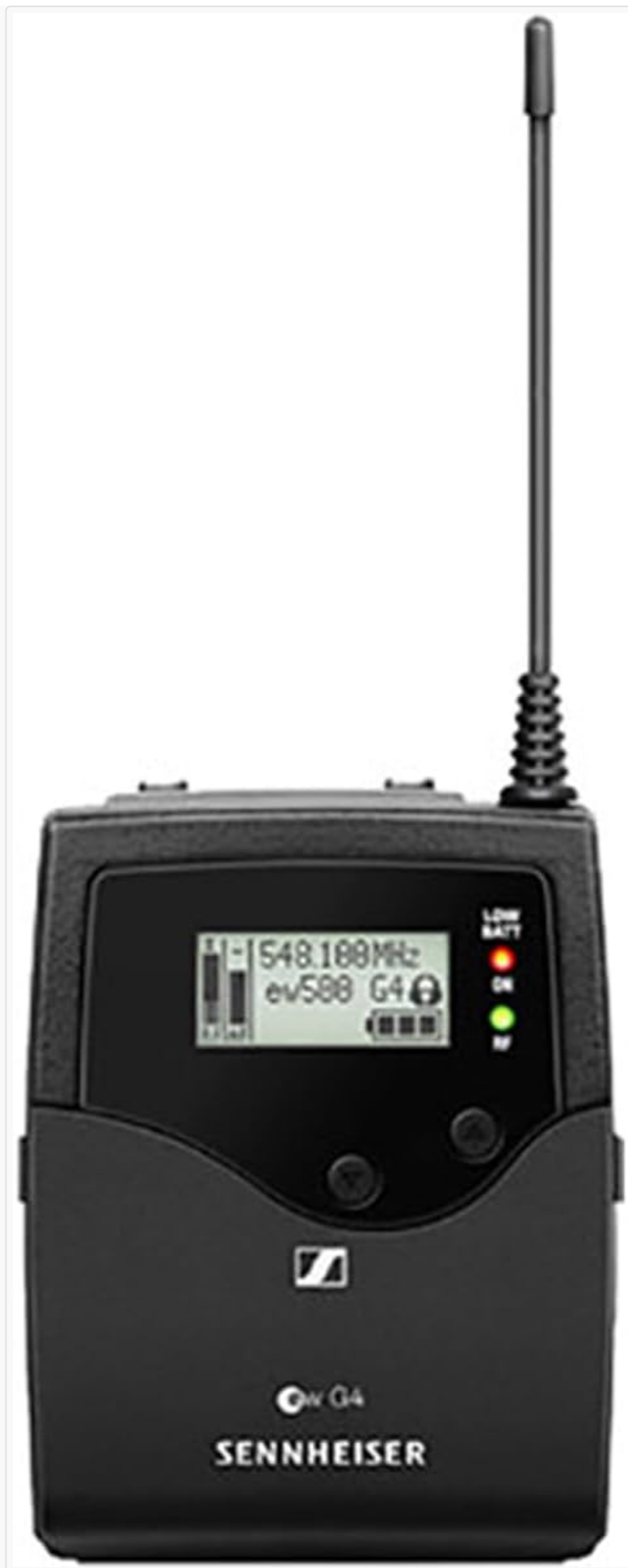
The image displays the Sennheiser EK 500 G4-AW+ portable camera receiver, showing its compact design, display screen, control buttons, and detachable antenna. This unit is designed for on-camera mounting.
