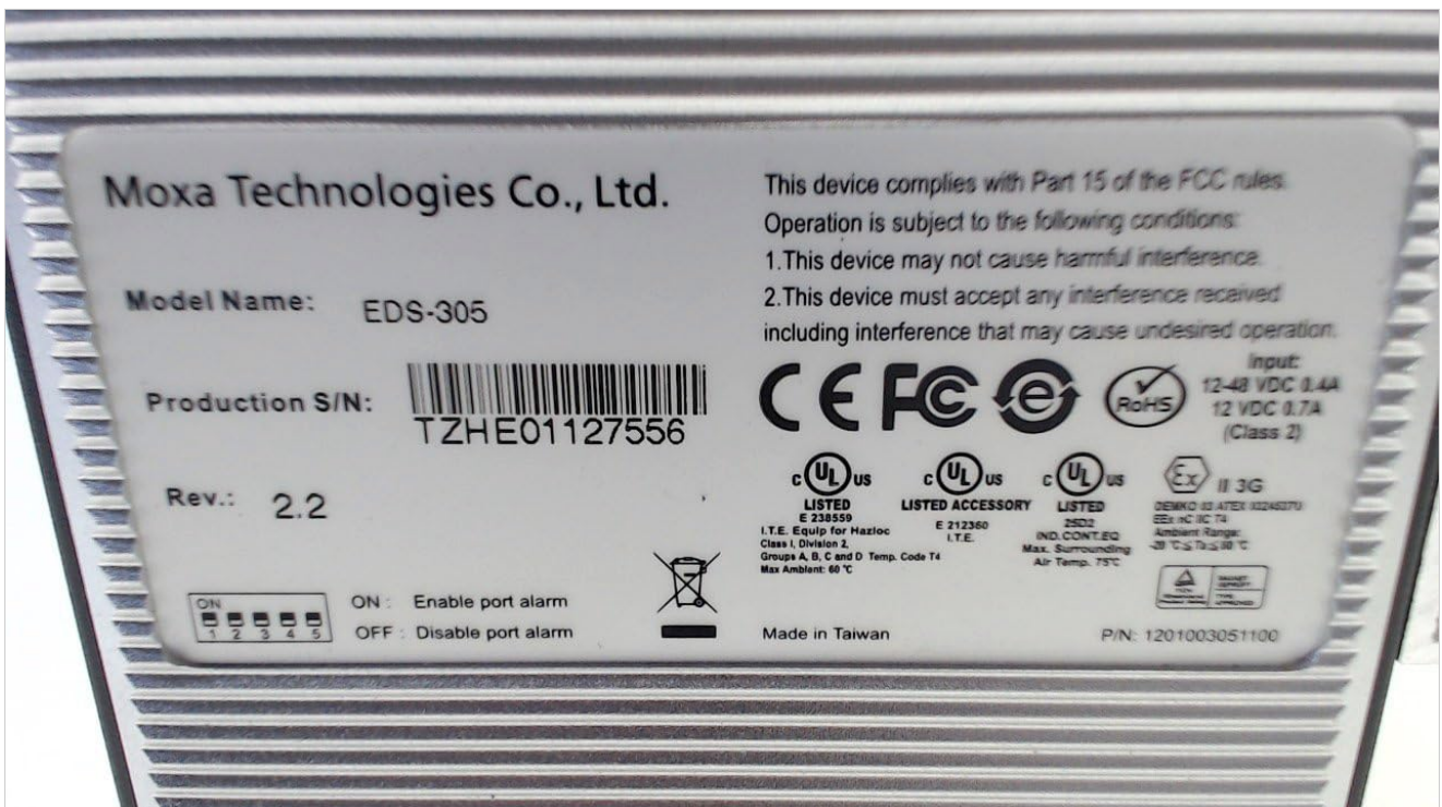
Figure 3: Bottom view of the Moxa EDS-305 switch. This image displays the product label with the model name 'EDS-305', production serial number, and various certifications (CE, FCC, UL, RoHS). It also clearly shows the input power specifications (12-48
