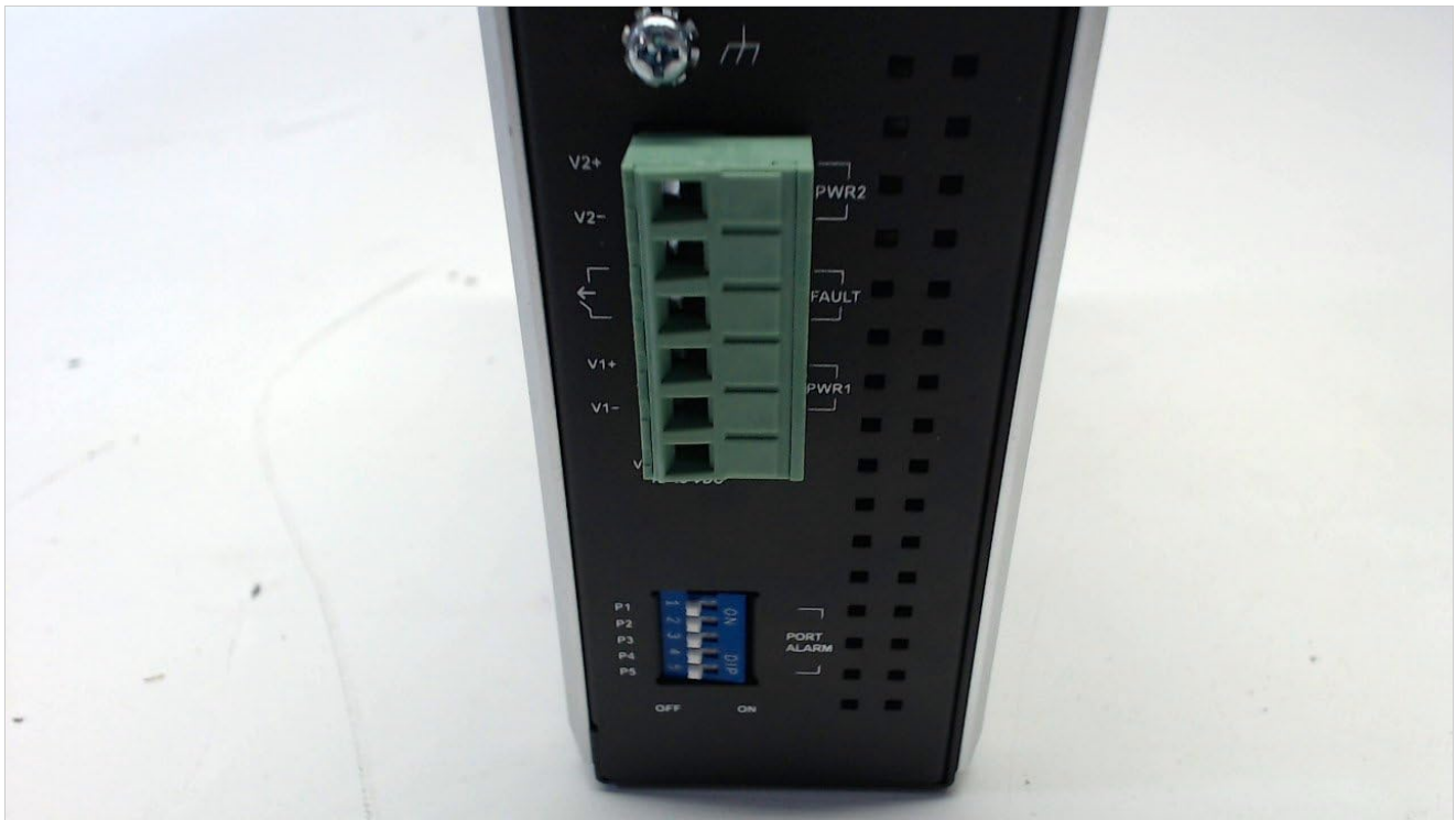
Figure 2: Rear view of the Moxa EDS-305 switch. This image shows the green terminal block for power inputs (V1+, V1-, V2+, V2-) and the fault relay output. Below the terminal block, a set of blue DIP switches labeled P1 through P5 and 'PORT ALARM' are visible, used for configuring port alarm settings.
