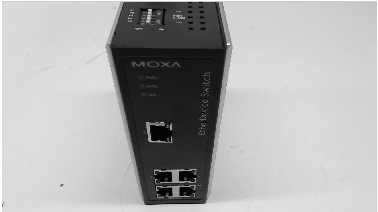
Figure 1: Front and side view of the Moxa EDS-305 switch. This image displays the device's front panel with PWR1, PWR2, and FAULT LED indicators, along with five 10/100BaseT(X) Ethernet ports. The Moxa brand logo is visible on the side.
