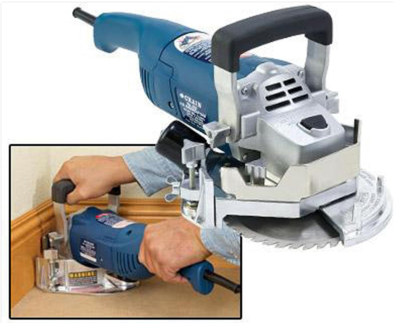
Figure 4.1: The Crain No. 835 Undercut Saw positioned for undercutting a wall, demonstrating proper handling.
