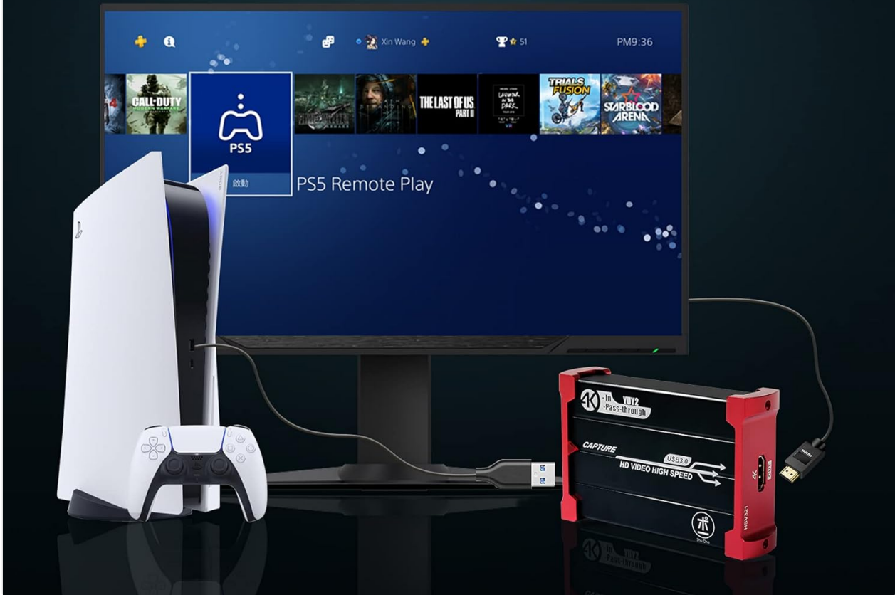
Image 5.2: PlayStation 5 connected to the Mirabox HSV321 for zero-latency HDMI passthrough. The image shows a PS5 connected via HDMI to the capture card, which then connects to a monitor and a laptop for streaming.
