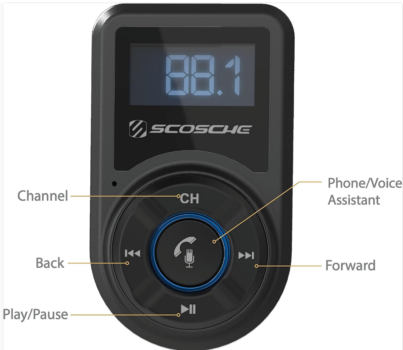
Figure 5: Labeled controls for Channel, Phone/Voice Assistant, Back, Forward, and Play/Pause.
