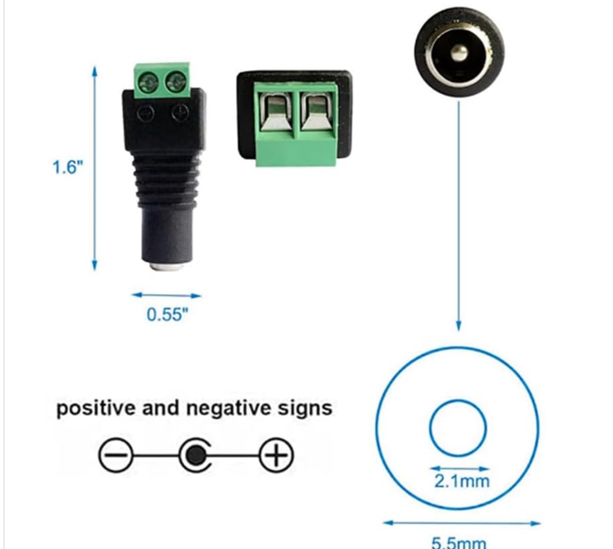
Figure 3: Female Connector Specifications (5.5mm x 2.1mm).
