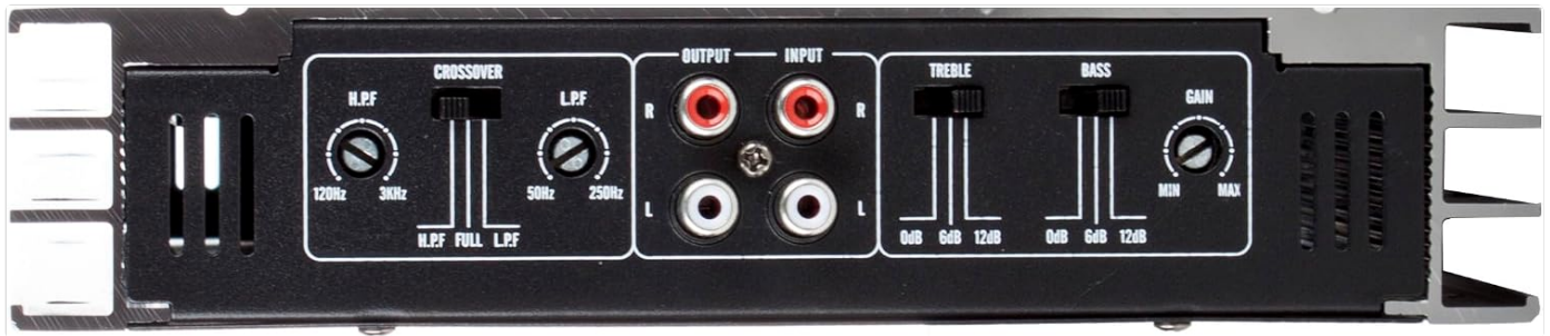
Figure 4: The side panel of the Excalibur X600.2 amplifier, showing the adjustable crossover (HPF/LPF), input/output RCA jacks, treble, bass, and gain controls.
