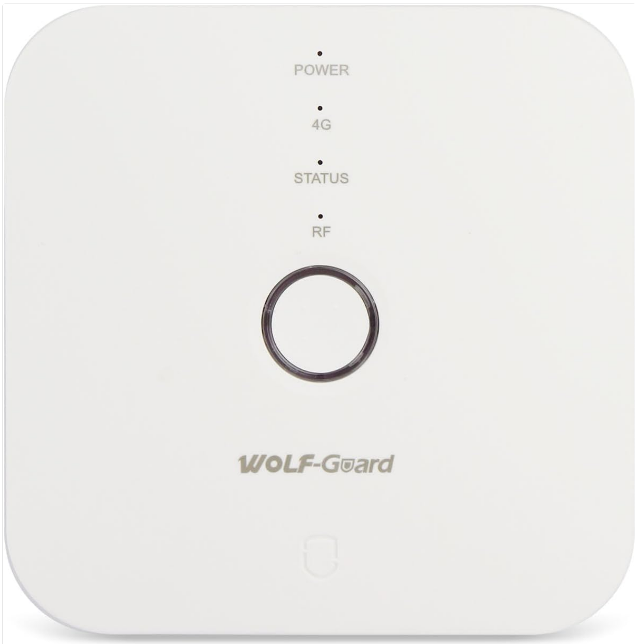
Figure 3.1: Top view of the alarm host, showing LED indicators for Power, 4G, Status, RF, and the central SOS button.
