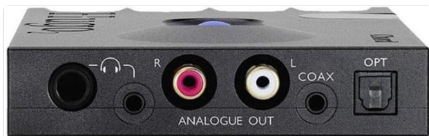
Figure 3: Rear panel of the Hugo 2, displaying the analog RCA outputs (left and right), coaxial digital input, and optical digital input. Also visible are the 3.5mm and 6.35mm headphone jacks.
