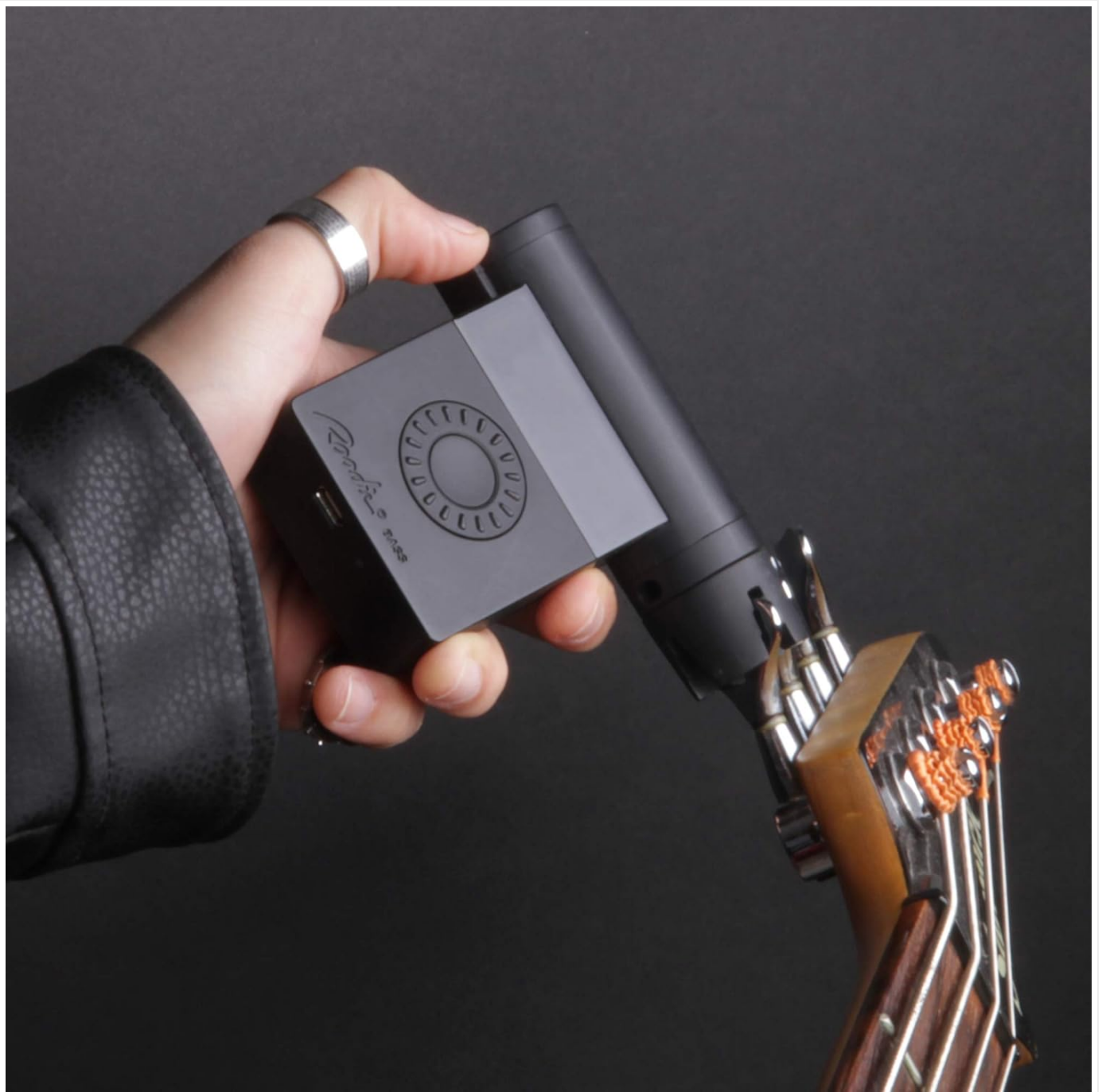
Proper placement of the Roadie Bass on a tuning peg for automatic tuning.
