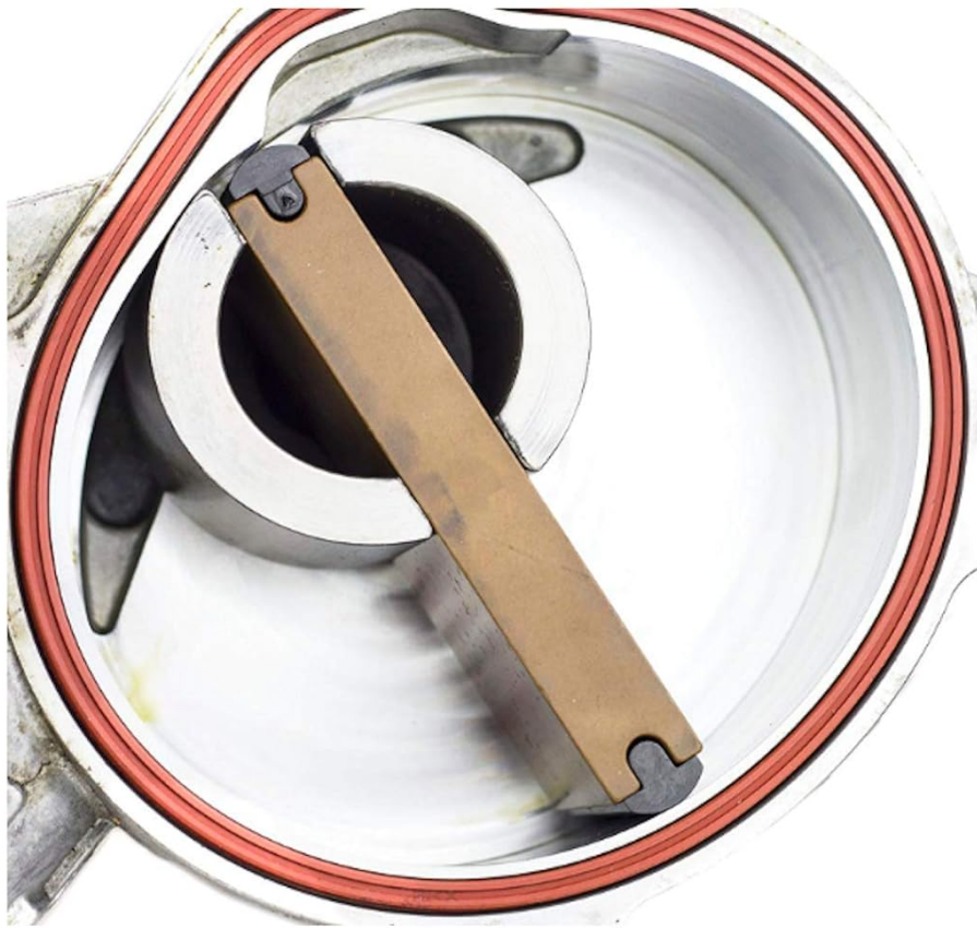
A detailed close-up showing a new brown O-ring correctly seated within the internal groove of a BMW vacuum pump housing. The internal rotor mechanism is visible, indicating proper seal placement during the resealing process.
