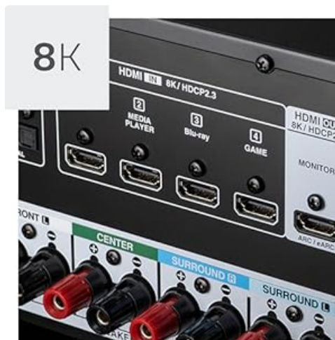
Figure 4: Close-up of the HDMI 8K/HDCP2.3 ports on a Denon AV Receiver, illustrating the advanced video connectivity options for high-resolution content.
