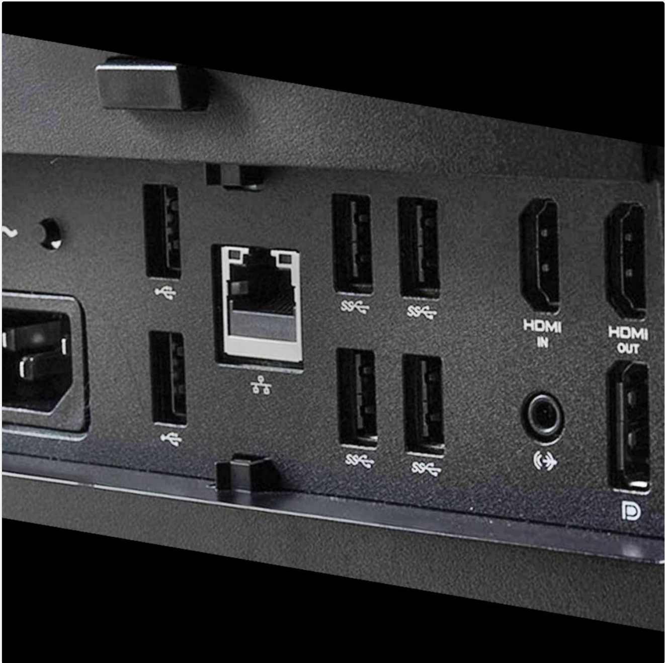
Figure 2.2: Detailed view of the rear ports on the Dell Optiplex 9030, including USB, Ethernet, HDMI In/Out, and audio jacks.
