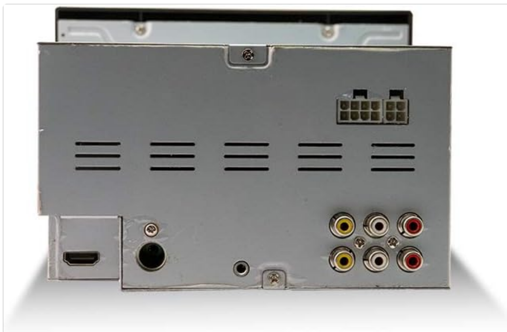
Figure 4: Rear view of the iRV Technology IRV31. This image shows the various input/output ports, including the main wiring harness connector, HDMI port, and RCA audio/video inputs and outputs, essential for proper wiring.
