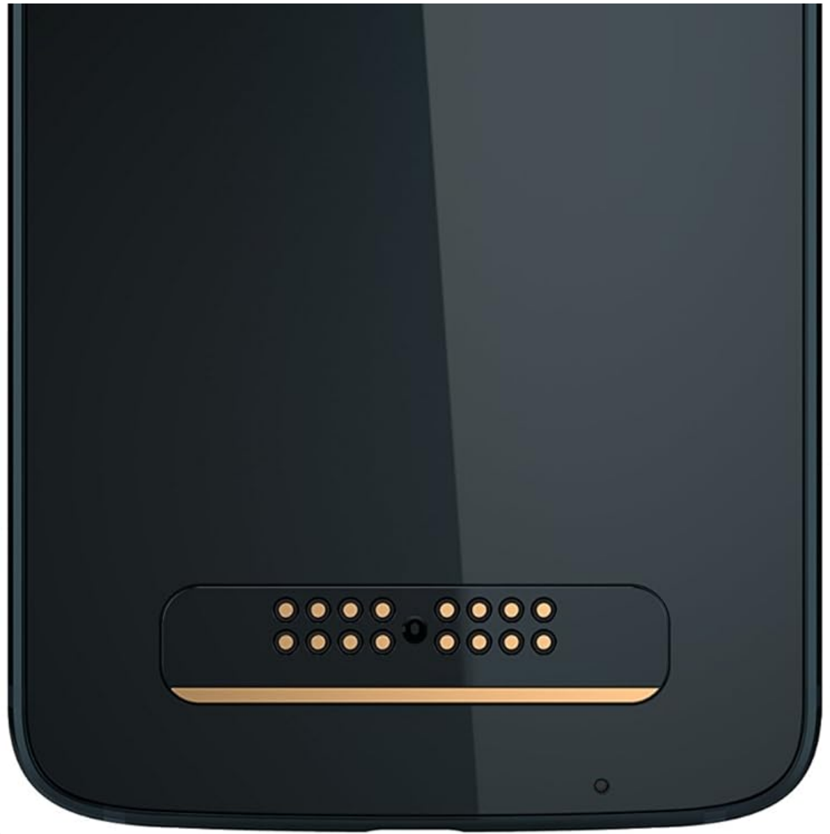
Figure 3.1: The back of the Moto Z3 Play, highlighting the magnetic connector pins for Moto Mods.
