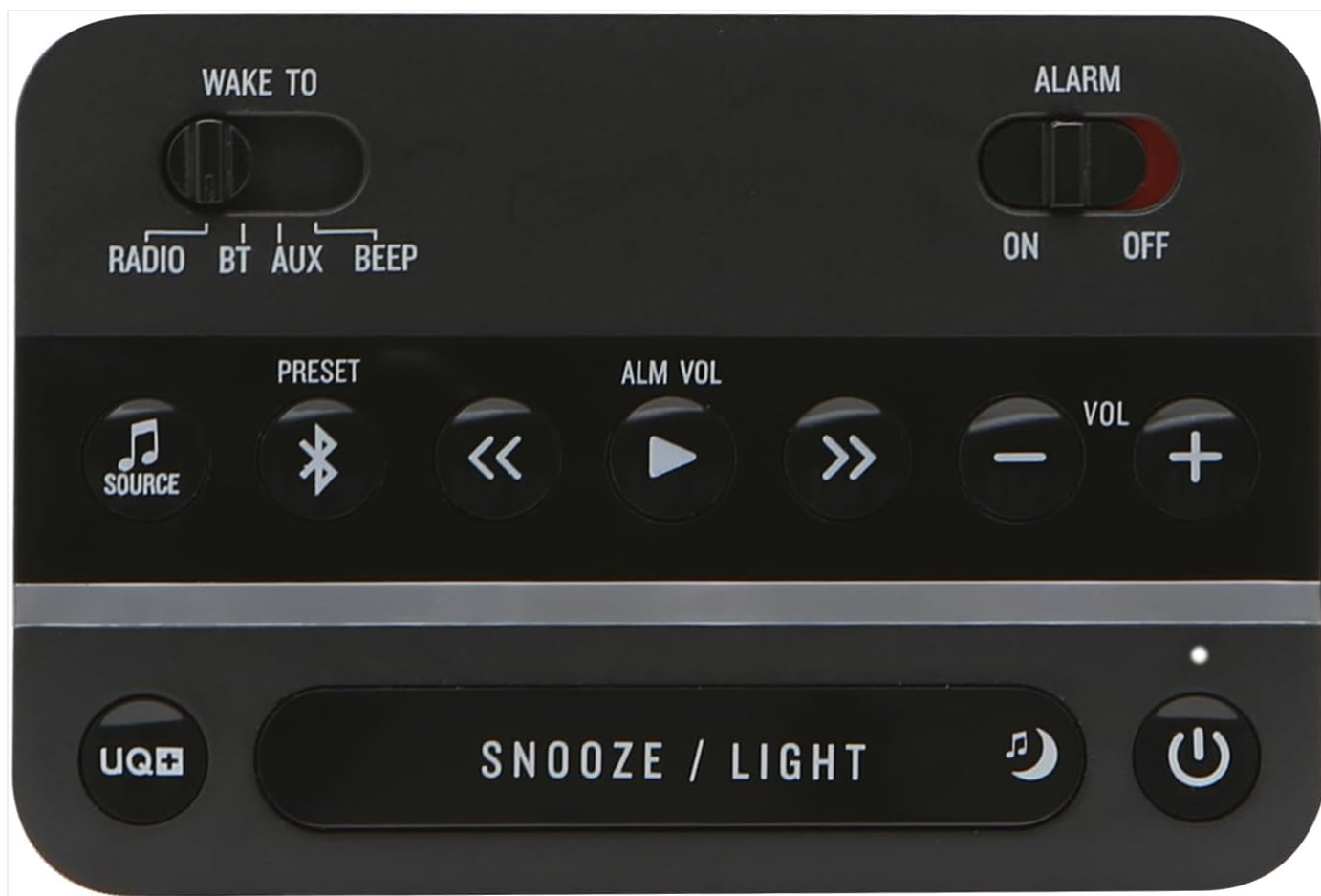
Figure 2: Top Control Panel. This image provides a detailed view of the top control panel. From left to right, there are switches for "WAKE TO" (RADIO, BT, AUX, BEEP) and "ALARM" (ON, OFF). Below these are buttons for "SOURCE", "Bluetooth pairing", "PRESET", "ALM VOL" (previous track, play/pause, next track), and "VOL" (minus, plus). A large "SNOOZE / LIGHT" button is centrally located, flanked by a "UQ+" button on the left and a power button on the right.
