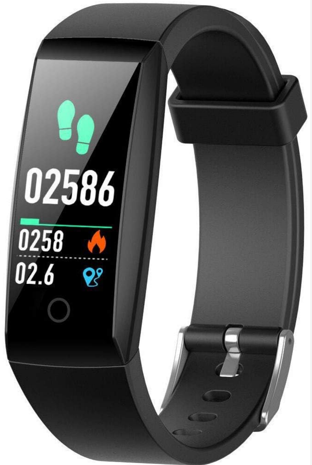
Figure 4.1: Front view of the HETP W8 Fitness Tracker displaying steps, calories, and distance.
