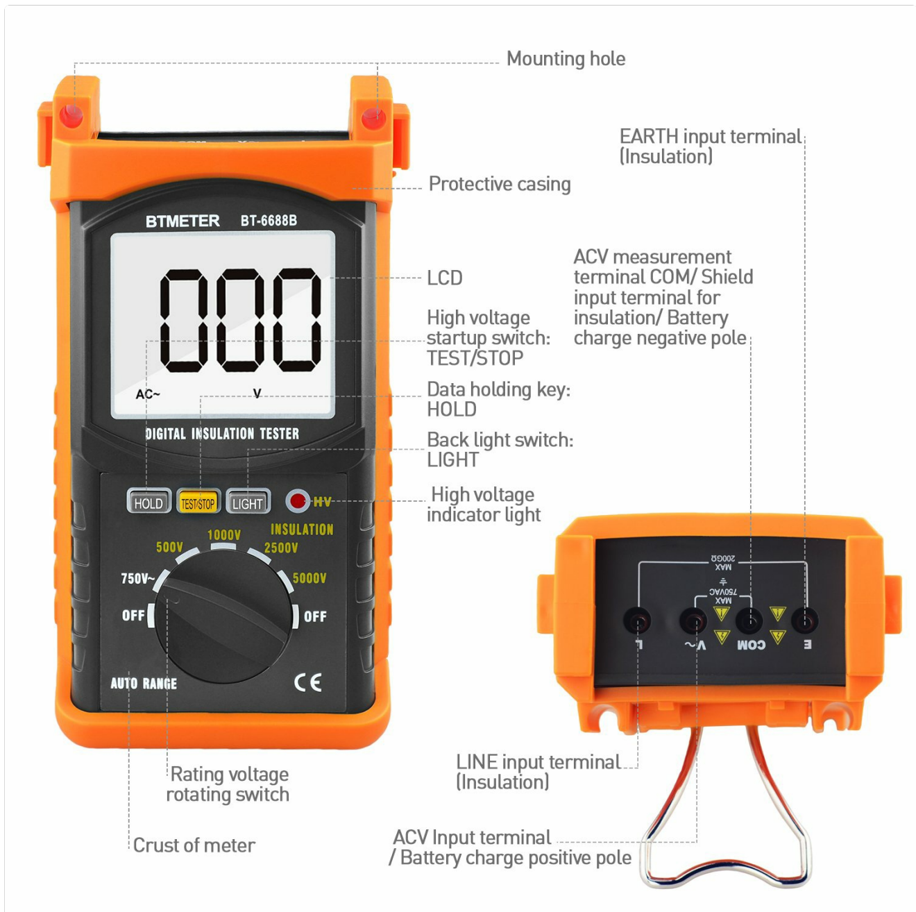
Image: Detailed diagram of the BT-6688B tester, highlighting the LCD, high voltage indicator, test/stop switch, data hold key, backlight switch, rating voltage rotating switch, input terminals (E, COM, V~, L), and protective casing.
