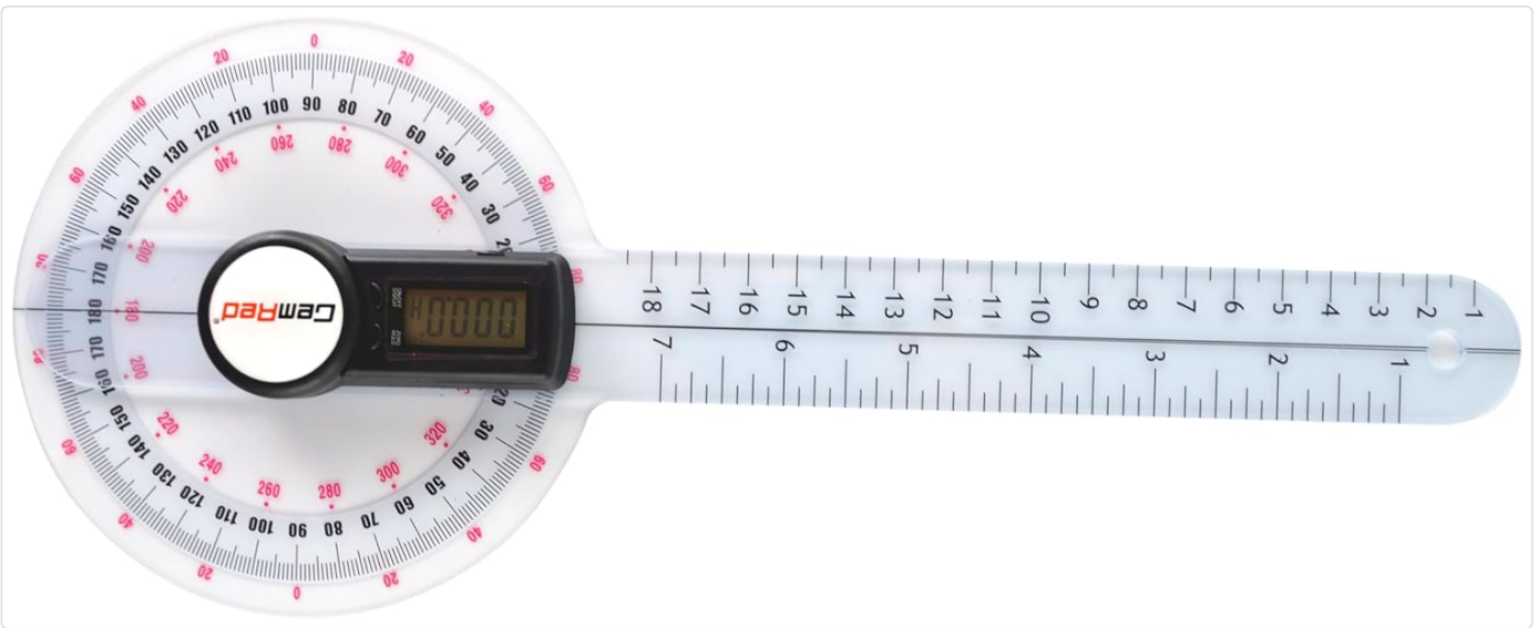
Figure 3.1: Front view of the GemRed Digital Angle Finder Goniometer 82311-00.
