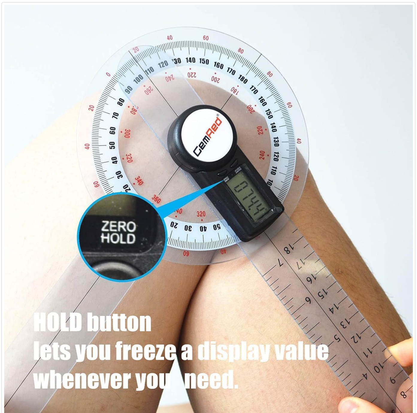
Figure 5.1: The ZERO HOLD button allows you to set a zero reference point and freeze the display value.
