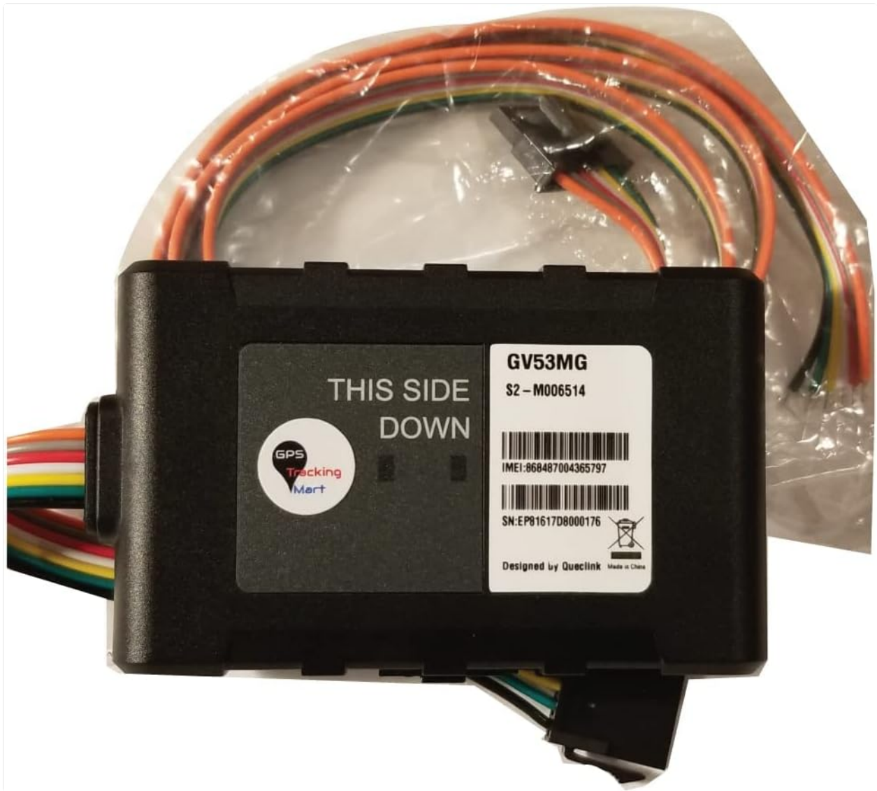
Image: The GV53MG device with its multi-colored wiring harness, indicating connection points.
