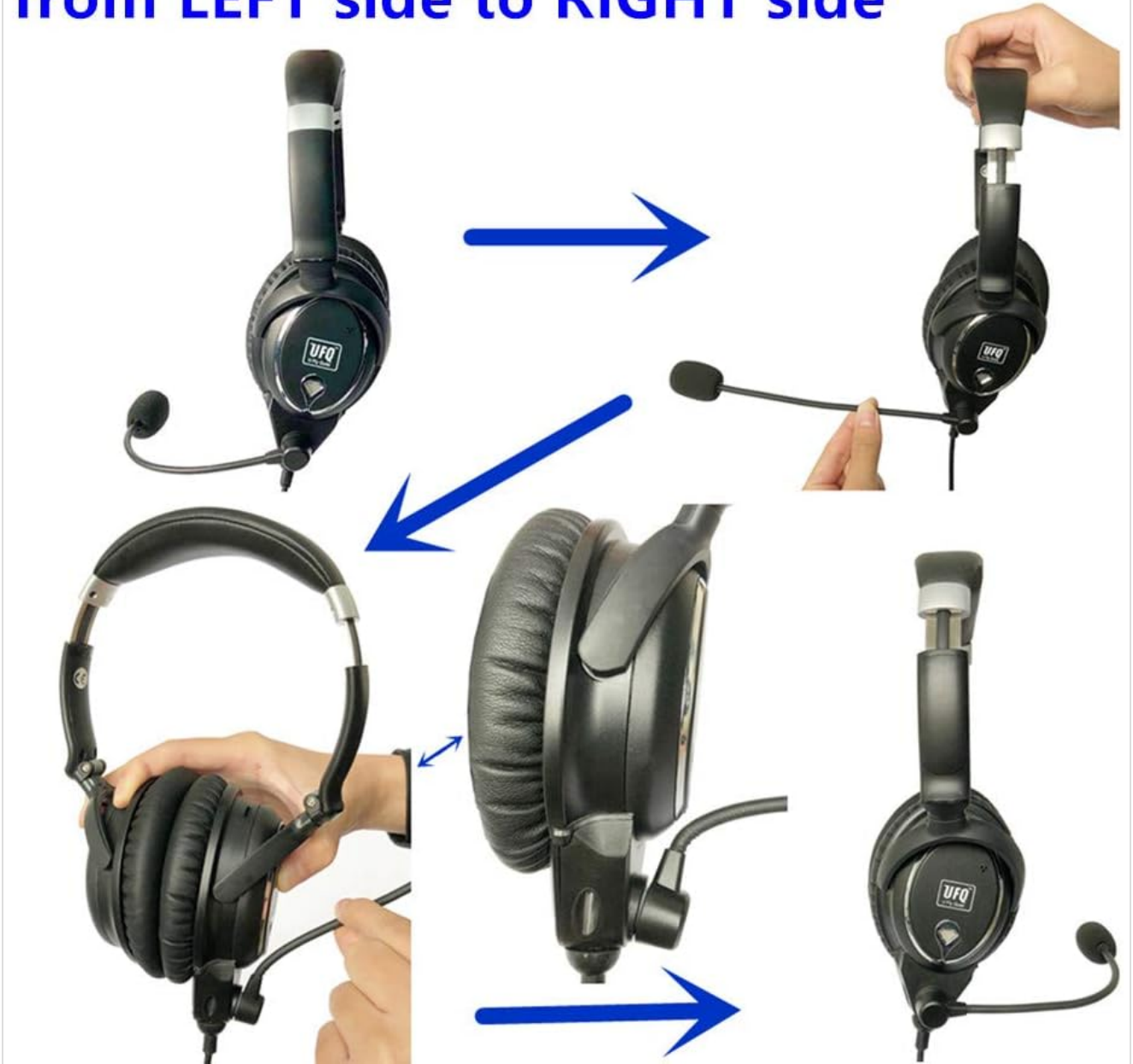
Figure 2.2: Visual guide demonstrating the 350-degree rotation capability of the microphone boom, allowing for flexible positioning on either side of the headset.
