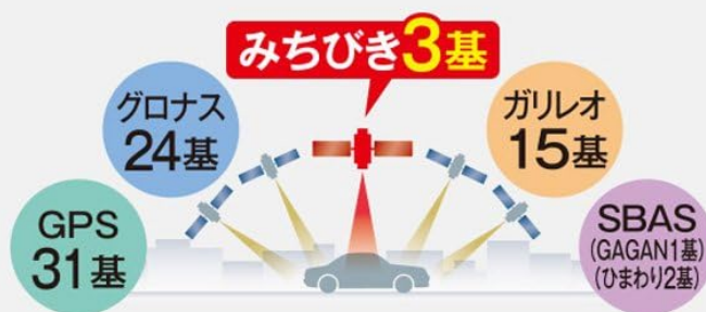
Figure 4: Diagram showing the Super GPS system, indicating the number of satellites from Michibiki, GLONASS, Galileo, GPS, and SBAS used for precise positioning.
