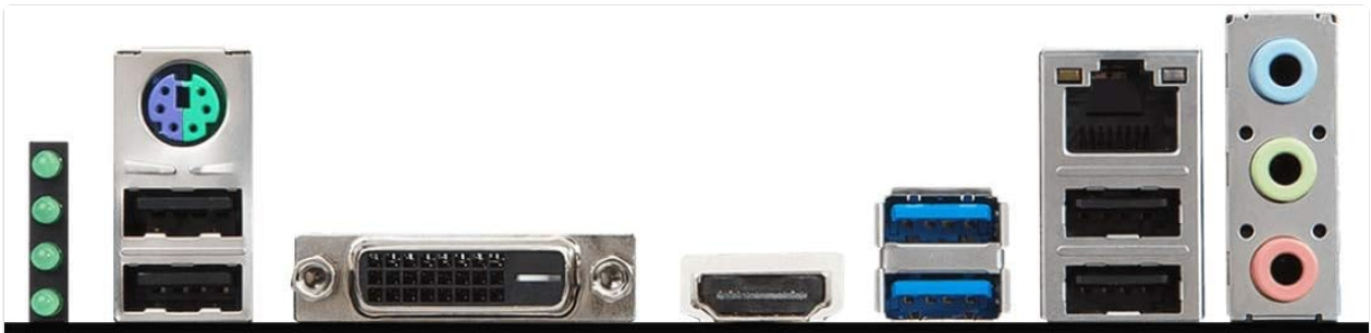
Figure 3: Rear I/O panel of the MSI B360-F PRO ATX Motherboard, showing various USB, display, and audio ports.
