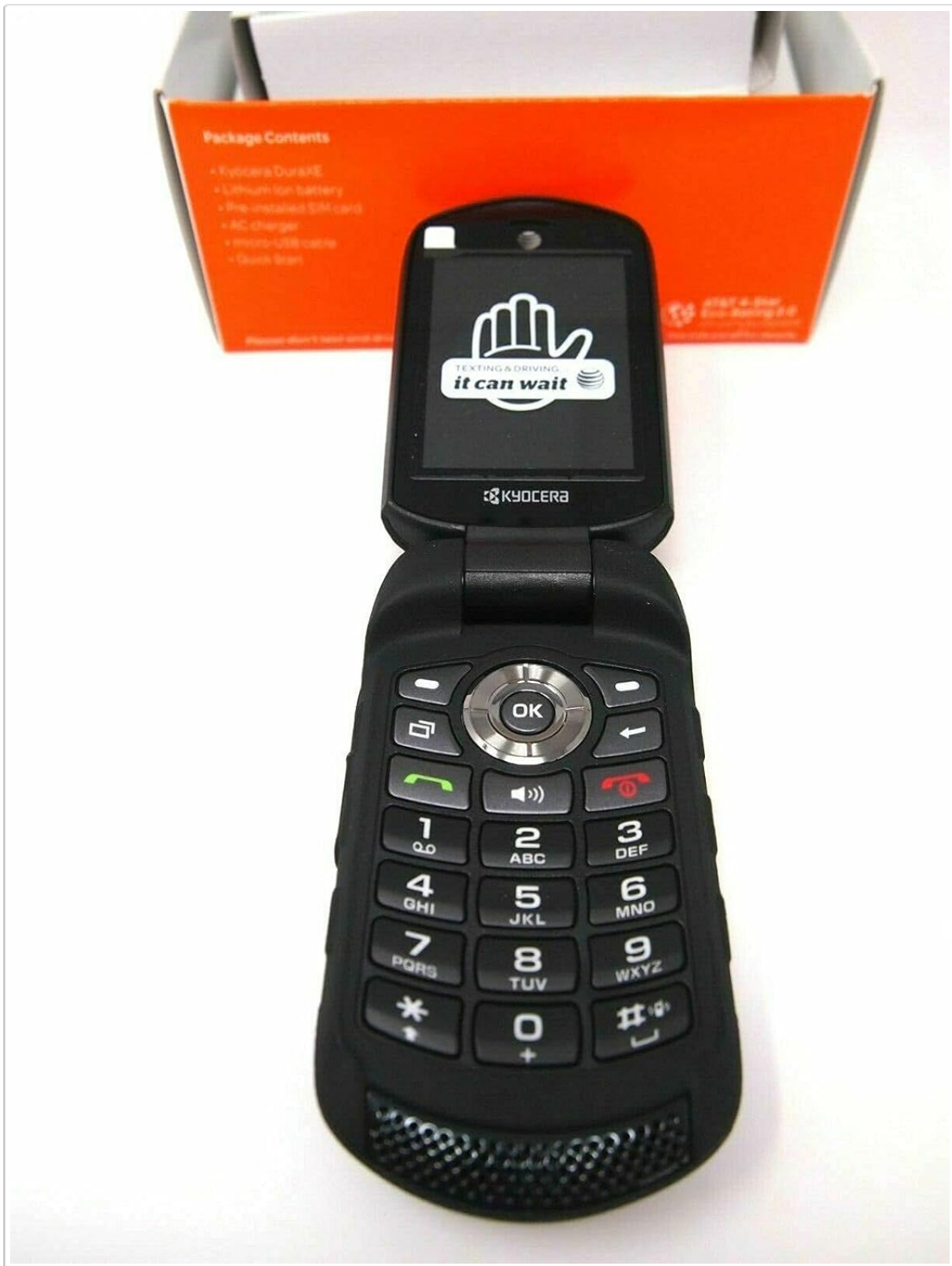
Figure 3.3: The Kyocera Dura XE E4710 flip phone in an open position, revealing the internal screen and the full keypad with navigation buttons.
