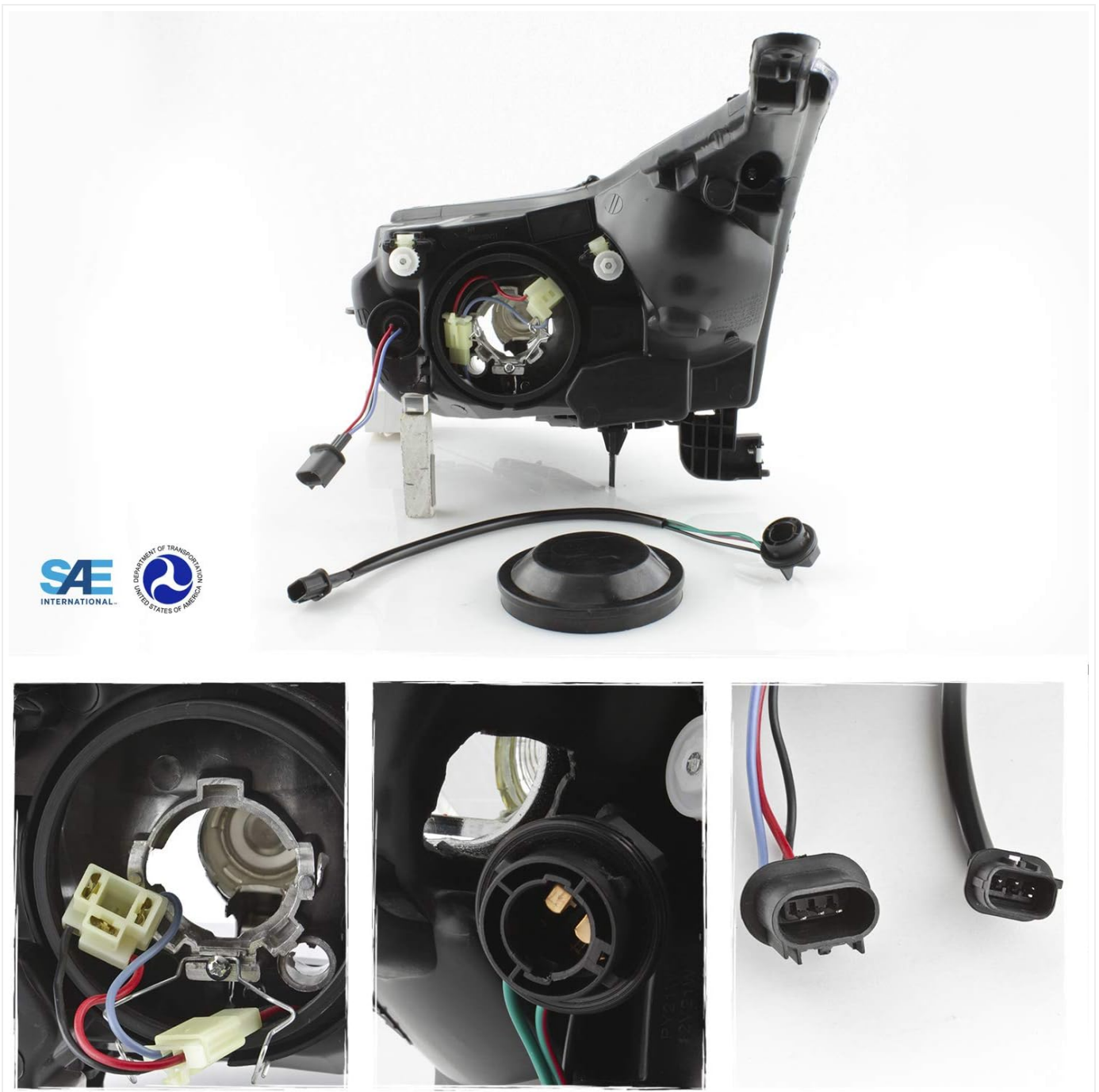
Image: The complete AKKON headlight assembly, showcasing its design and compliance with SAE and DOT standards.
