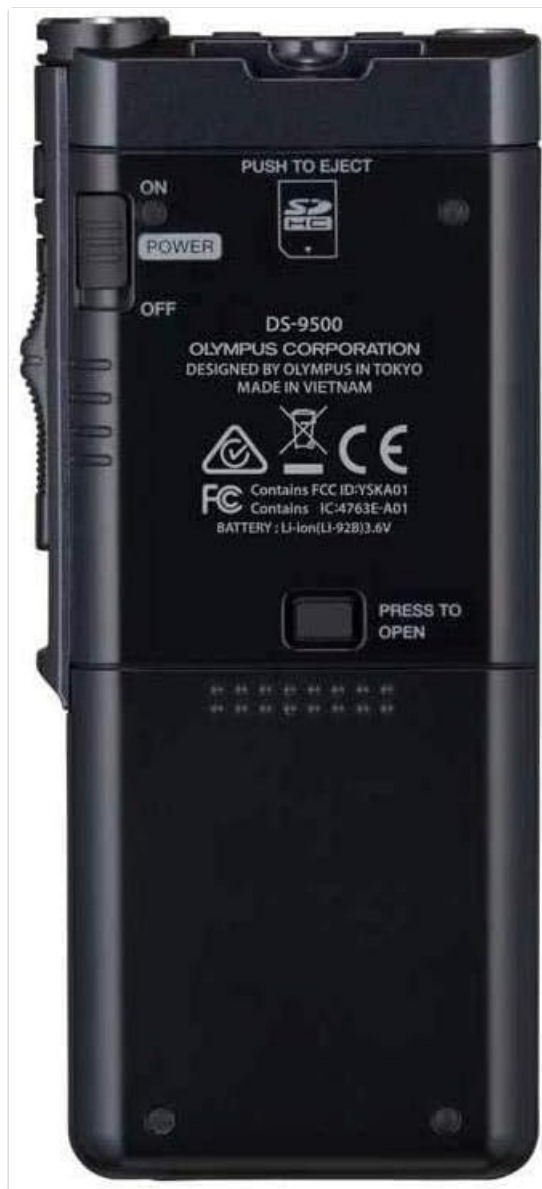
Figure 2.2: Back View. The rear of the DS-9500 features the power switch (ON/OFF), a 'PUSH TO EJECT' mechanism for the SD card slot, and the battery compartment release. Model information and regulatory markings are also visible.
