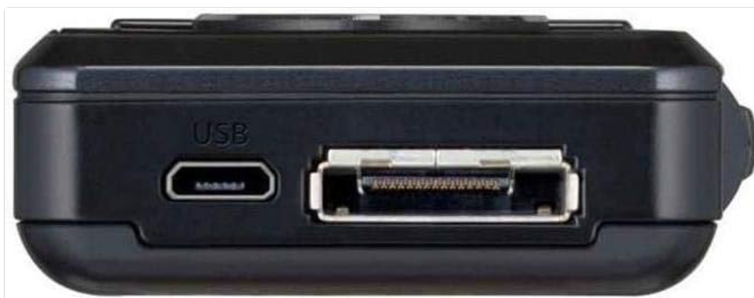
Figure 2.5: Bottom View. The bottom of the device includes the USB ports for charging and data transfer, facilitating connectivity with a computer or docking station.
