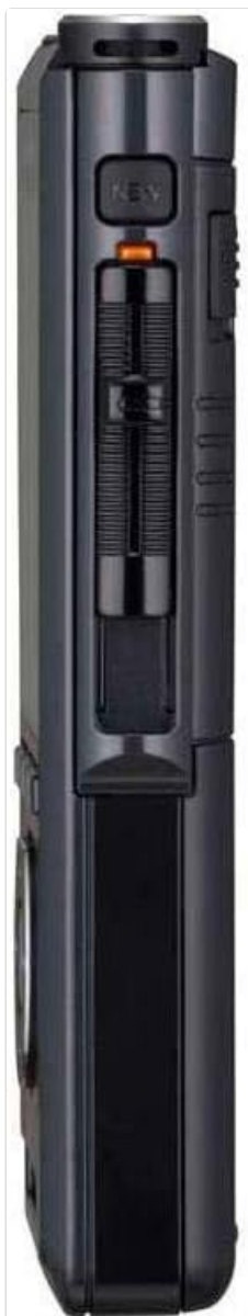
Figure 2.4: Right Side View. The right side of the DS-9500 features the optical slide switch, a key control for recording, stopping, and playback functions, designed for tactile and reliable operation.
