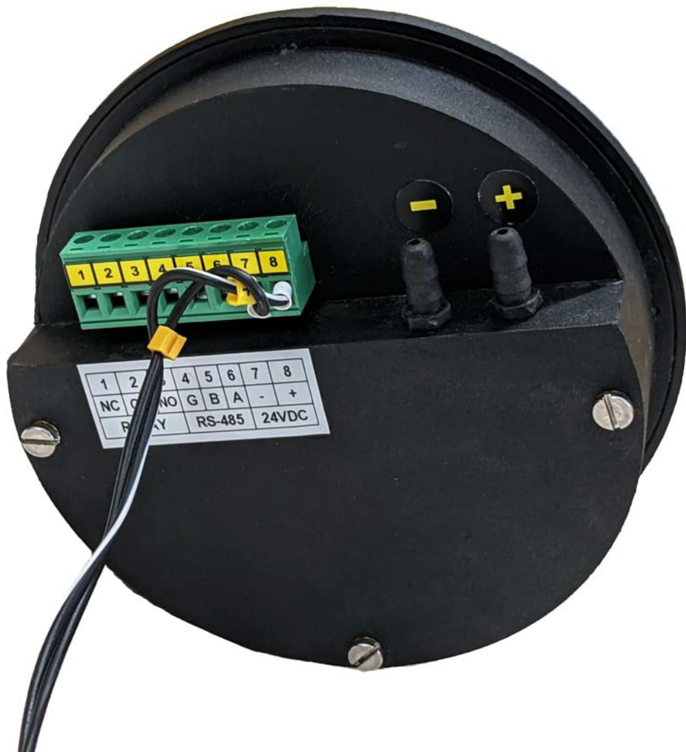
Figure 4: Rear view of the controller, detailing the power input terminals, hose nipples, and optional communication/output terminals.
