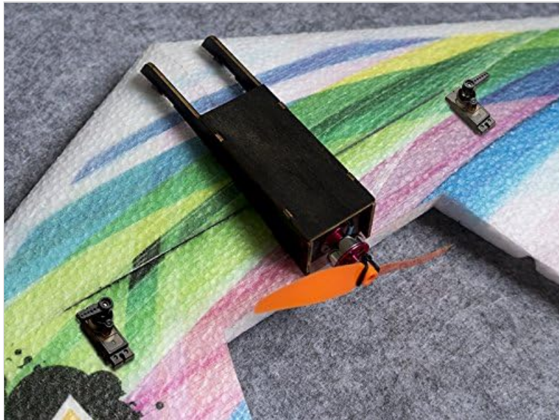
Figure 4.2: Motor and servo installation. This image illustrates the placement of the small electric motor and two servos within the foam structure of the flying wing.
