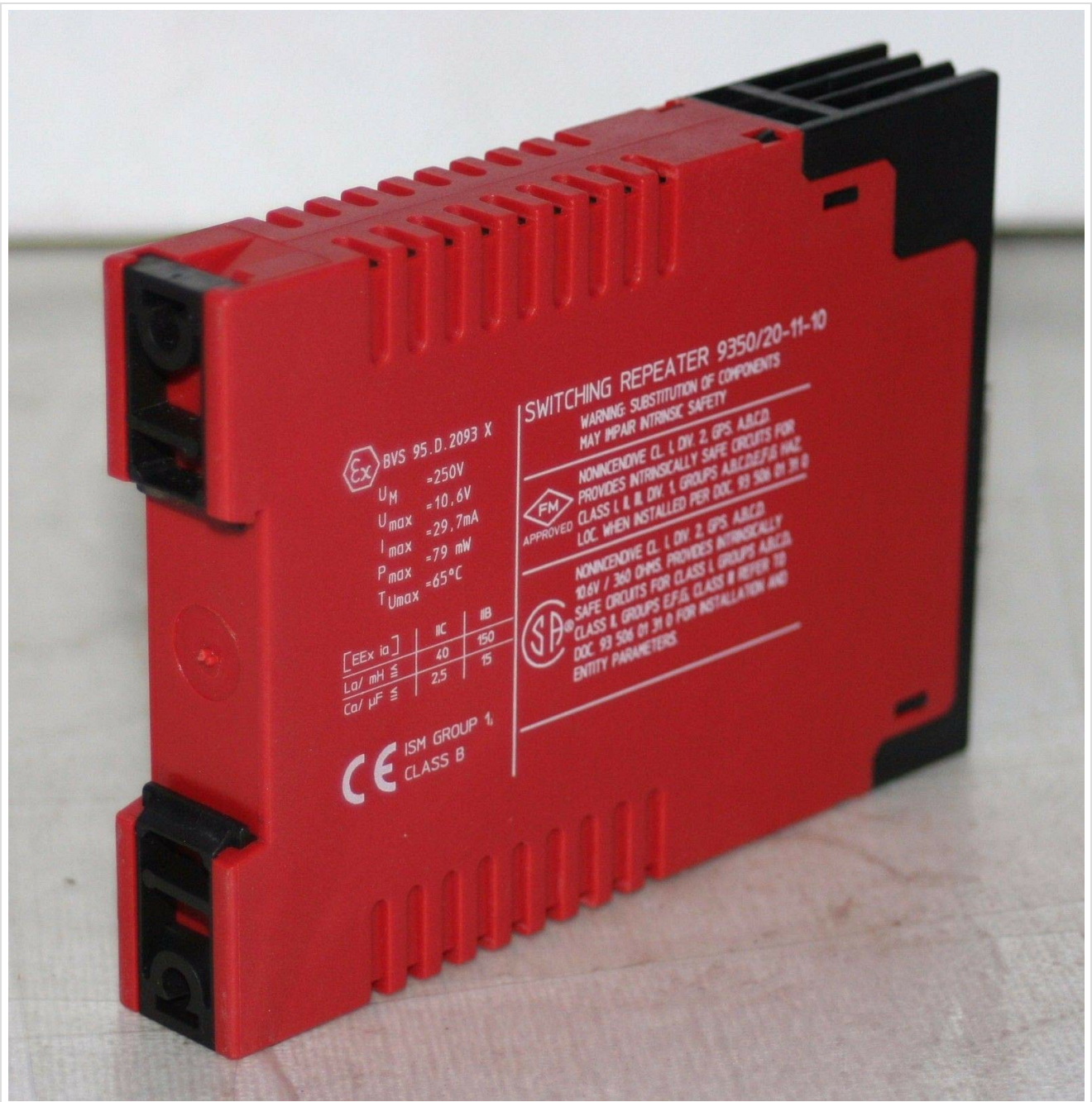
Figure 3.2: Side view of the module, displaying key safety certifications and electrical parameters such as U_M , U_{max} , I_{max} , P_{max} , and T_{Umax} .
