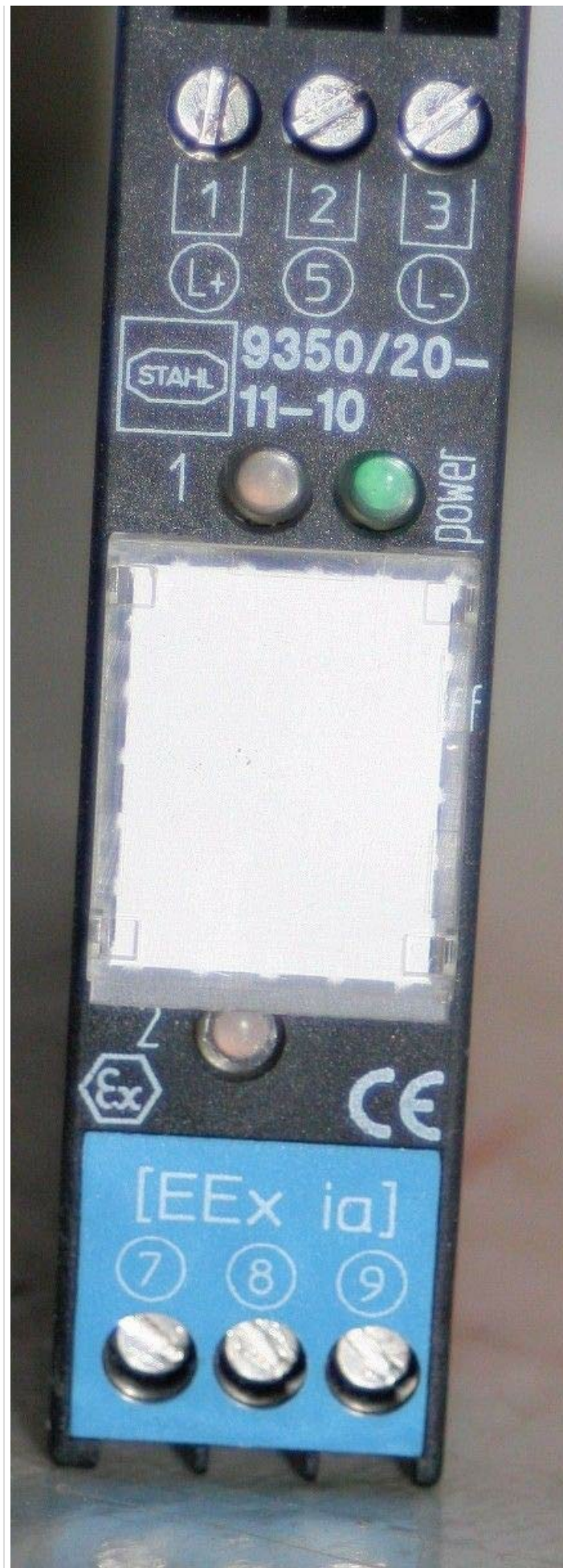
Figure 3.3: Close-up view of the terminal blocks and indicator lights on the module. Shows connections for L+, L-, and intrinsically safe circuits.
