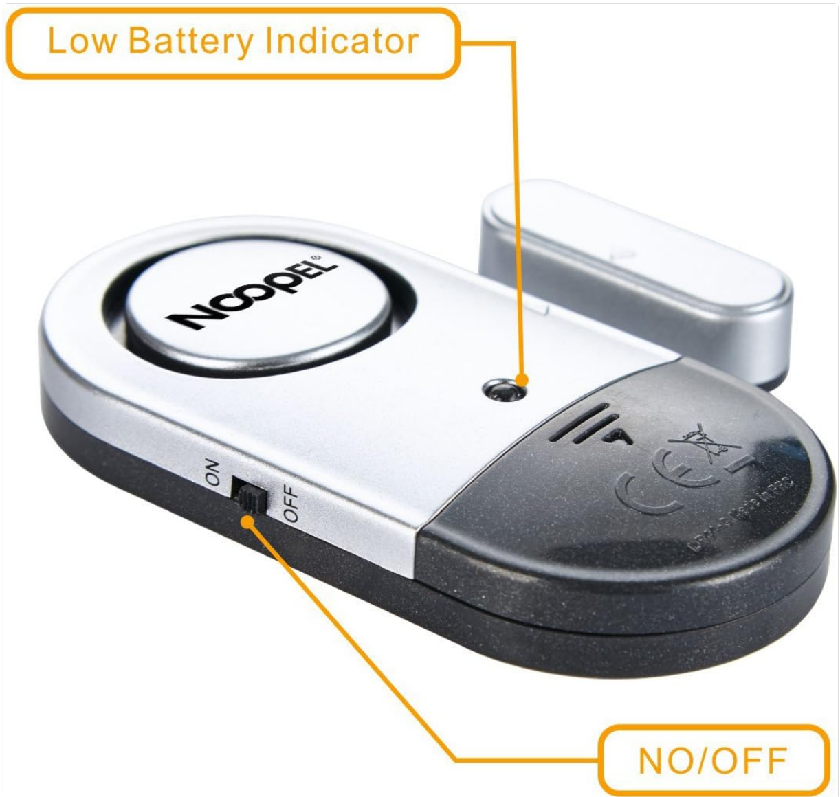
This close-up view of the Noopel Door Window Alarm highlights its key controls. A small black switch labeled 'ON' and 'OFF' is visible on the side of the main unit, used to activate or deactivate the alarm. Above the switch, a small LED light is indicated as the 'Low Battery Indicator,' which will alert the user when batteries need replacement.
