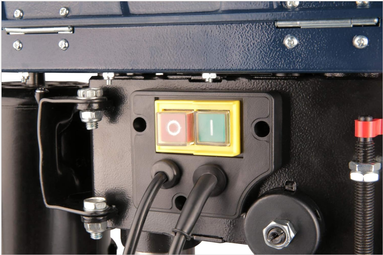
Image 4: The main power switch with green 'on' and red 'off' buttons.
