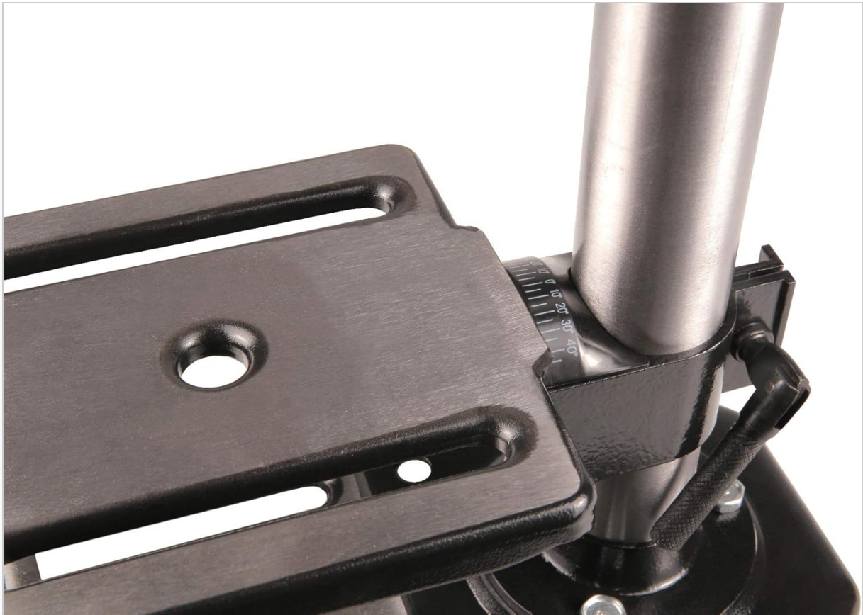
Image 2: Close-up of the adjustable work table and its angle indicator.
