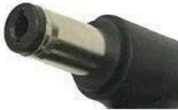
Image 3.2: A close-up view of the barrel connector, which plugs into the compatible device's power input port.
