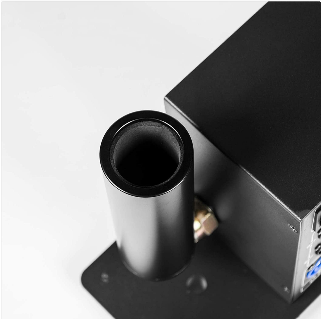
Figure 6: Inspect the CO2 nozzle for cleanliness and obstructions.
