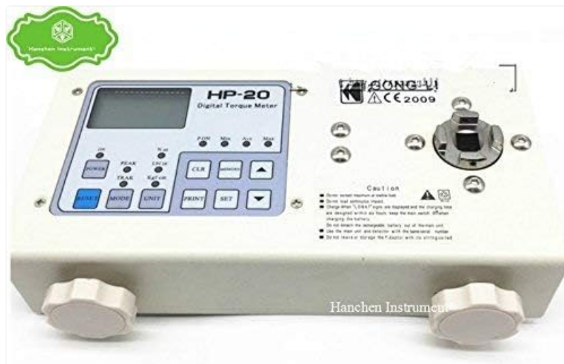
Figure 3.1: Detailed view of the Hanchen HP-20 control panel and display.
