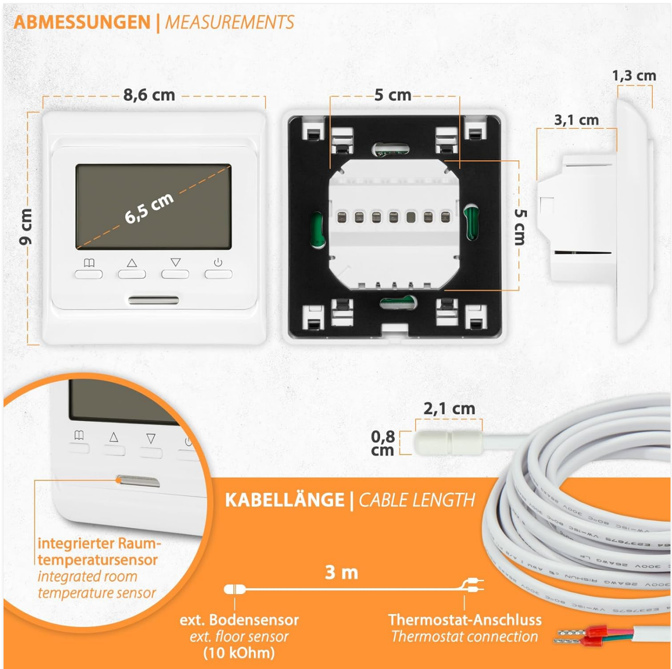
Figure 4.2: Dimensions of the E51 Digital Thermostat and cable lengths for the integrated room temperature sensor, external floor sensor, and thermostat connection.
