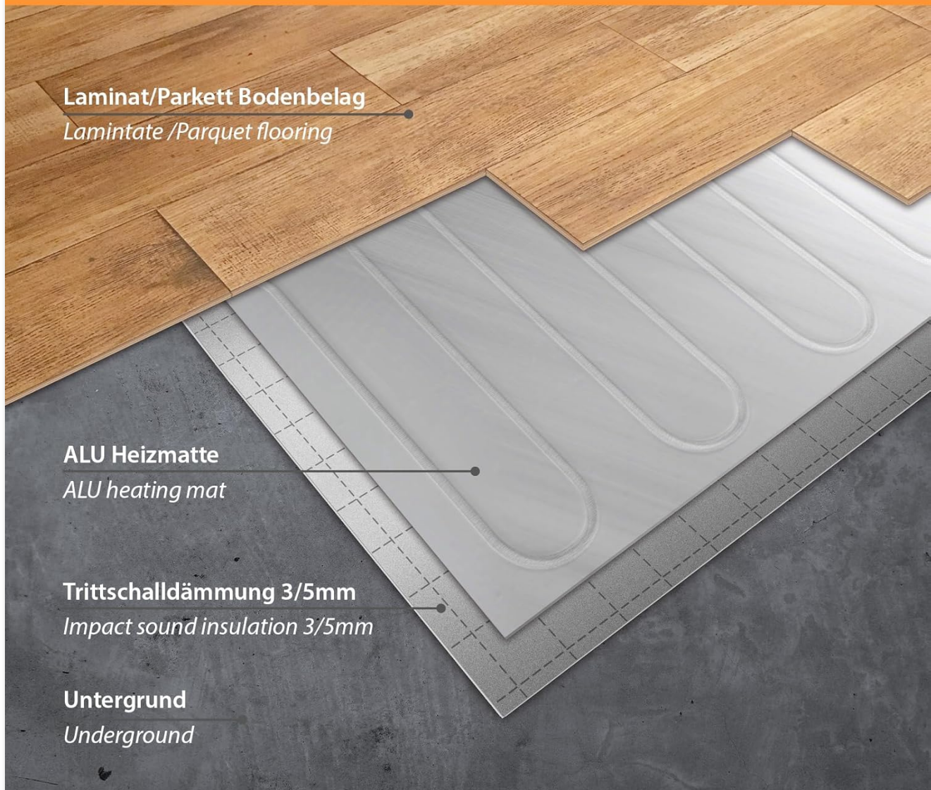
Figure 5.1: Diagram illustrating the layers of an electric underfloor heating installation, showing the underground, impact sound insulation, ALU heating mat, and laminate/parquet flooring.
