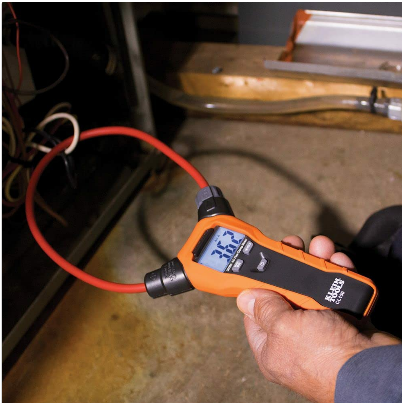
Figure 3: Demonstrating the use of the flexible clamp in confined areas.
