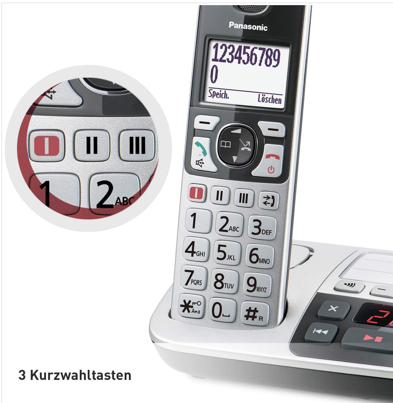
Image: A detailed view of the handset's upper keypad area, showing the three programmable quick dial keys (I, II, III).
