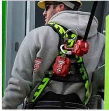
Image 2.1: Proper placement of the dorsal D-ring on the back.
